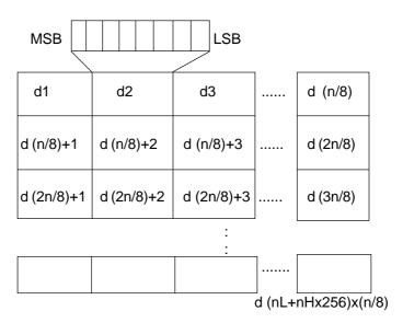
Defines Command: GS \* xy [d1] ... [d]x X y X 8
