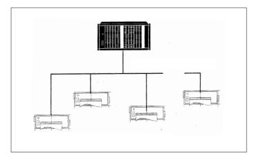
Each printer is addressable, which allows the connection of up to 31 devices to one sender device via a data line at the RS 485 interface, e.g. to a PLC.
