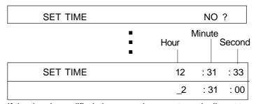
If the time is modified, the seconds are automatically set to zero.
