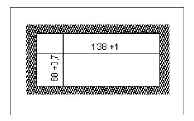
The IPP 144 - 40 G fits into a DIN standard panel cut out. It is inserted into the switchboard opening from the front side and is fixed against the switchboard rear using mounting screws. The switchboard thickness must not exceed 12 mm.
