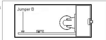
If the jumper B is connected, the "MENU / SELECT" key is locked; menu parameters can neither be printed or modified.
