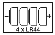
Fig. 5.1. Correct battery placement
