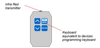
InfraRed remote controller type **SIR-15** may be used as external programming keyboard for all made by SIMEX devices equipped with IR receivers, and remote programming functions. Pressing of any local IR controller key, causes transmission of it's code to the device. Functions of particular keys depend on devices features and are described in their manual.
