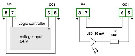
Figure 4.15. Example of OC-type outputs connection
