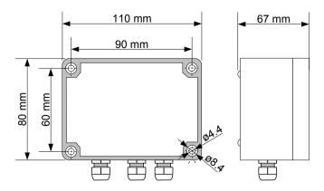
Figure 4.1. Device and assembly dimensions
