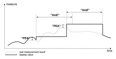
Figure 6.1. Process of peaks detection
