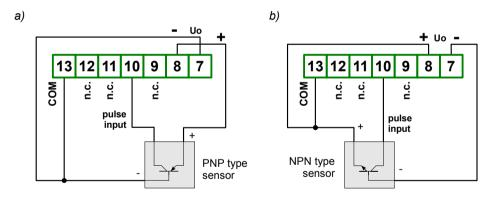
Figure 4.14. An example of sensor connection:
