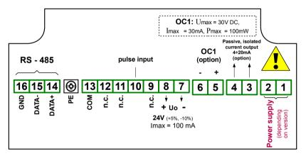
Figure 4.10. Terminals description (OC-type and passive current outputs)
