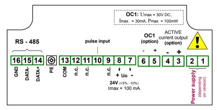
Figure 4.9. Terminals description (OC-type and active current outputs)
