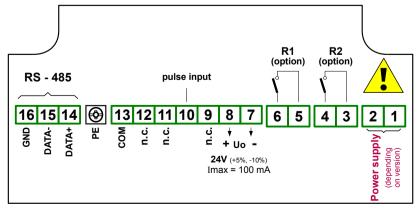
Figure 4.4. Terminals description (relay outputs)
