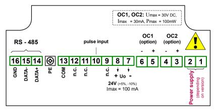
Figure 4.5. Terminals description (OC-type outputs)
