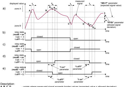
A. B. C. D - points where measured signal exceeds border values (expected value ± allowed deviation)
