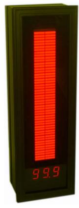
The gauge is enclosed in Aluminum Cabinet and supplied from 24VDC or 115/230VAC. The programming keys are at the main board and are accessible after removing the rear panel. Optional Keyboard can be plugged into the RS485 D-SUB at the rear panel.
