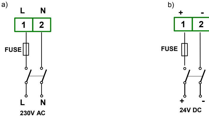
Figure 4.6. Connection of power supply a) for 230V AC version; b) for 24V DC version
