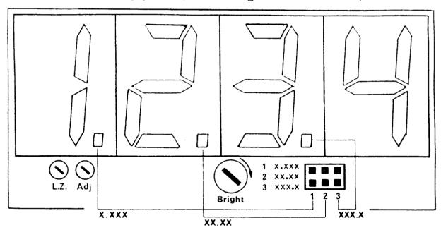
If no lighted decimal point is required, the jumper may be positioned as shown below:
