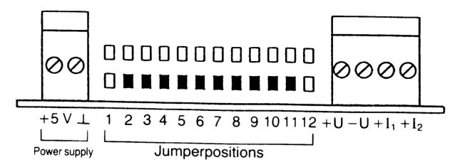
Note: Unused jumper links may be stored transversely in the lower positions marked in black between pins 2 and 11
