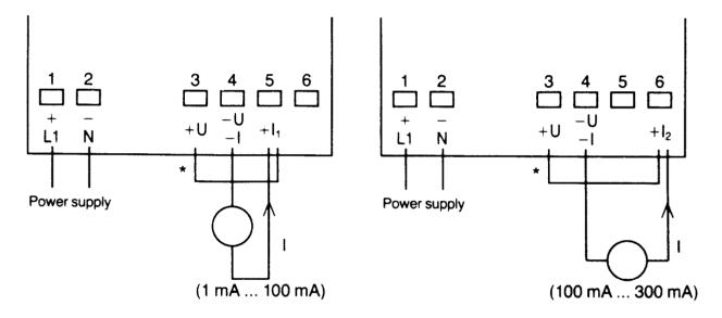
\*For **current measurement**, the user has to **externally link** terminals 3 (+ U) and  $5 (+ I_1)$ , or terminals 3 (+ U) and  $6 (+ I_2)$ . This link should be as short as possible and of low resistance.
