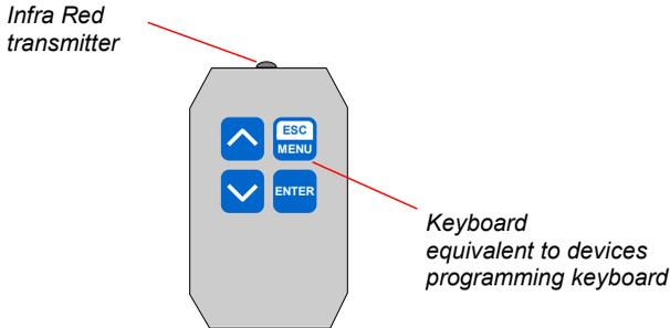
InfraRed remote controller type **SIR-15** may be used as external programming keyboard for all made by SIMEX devices equipped with IR receivers, and remote programming functions. Pressing of any local IR controller key, causes transmission of it's code to the device. Functions of particular keys depend on devices features and are described in their manual.
