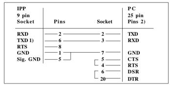
1) With ITT standard cable, this connection is made to pin 4.
