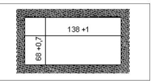
The IPP 144 - 40 G fits into a DIN standard panel cut out. It is inserted into the switchboard opening from the front side and is fixed against the switchboard rear using mounting screws. The switchboard thickness must not exceed 12 mm.
