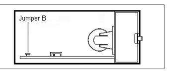
If the jumper B is connected, the "MENU / SELECT" key is locked; menu parameters can neither be printed or modified.
