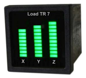
**Bargraph OCB30** with three green or red bars with 10 segments each is designed for monitoring of three independent signals 0-10V. The bargraph is supplied from 24VDC or 24VAC and is enclosed in a DIN cabinet 48 x 48mm. The depth behind the panel is 60mm. The three signal inputs and the supply voltage are connected via screw terminals.
