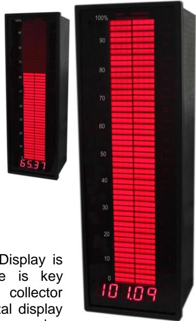
**OCB500** with 50 Bargraph Segments and a five digit high resolution Display is designed for connection to analogue process signals. The gauge is key programmable and permits settings of two Set Points with open collector Transistors or two mechanical Relays. In the measuring mode the digital display follows the input signal and permits high resolution of 16 Bits. In the programming mode the display shows the parameters.
