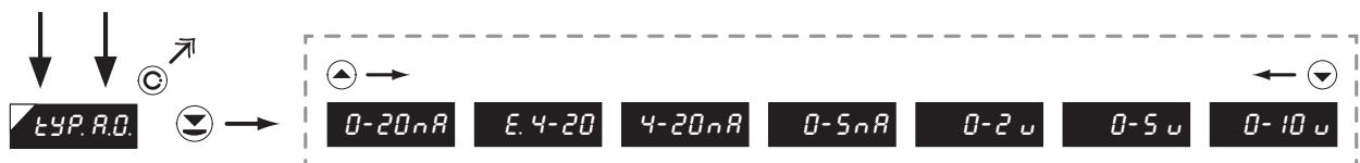
**TYP. A.O.** Setting the type of analog output
