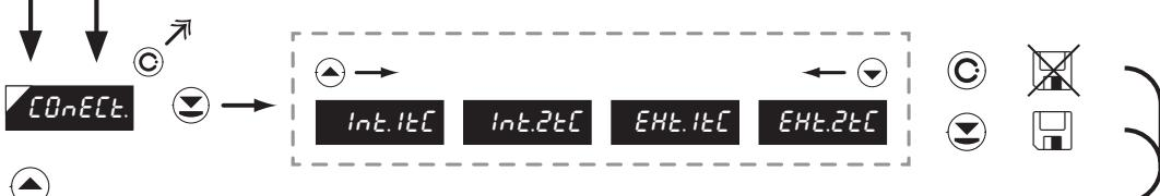
**CONNECT.** Selection of the type of sensor connection
