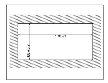
The IPP 144 - 40 fits into a DIN standard panel cut-out. It is inserted into the switchboard opening from the front side and is fixed against the switchboard rear using mounting screws.
