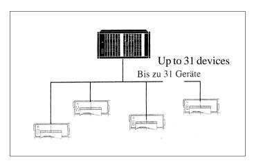
Each printer is addressable, wich allows the connection of up to 31 devices to one sender device via a data line at the RS 485 interface, e.g. to a PLC.
