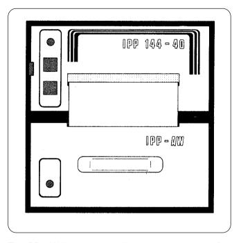
The IPP - AW is a paper reroll mechanism designed for use with the IPP 144-40. It has been designed to match the printer in colour and style. It is preferrably installed directly underneath the printer. The printed paper is automatically wound on a drum by a motor. A swivel front panel allows easy paper handling.
