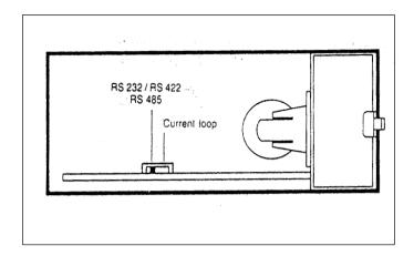
Slide snap lock to the right hand side, swivel front door out.
