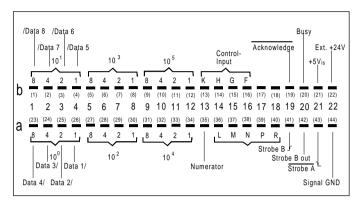
In BCD format 6 decades (pins 1a ... 12b), see chapter 4.1. connection diagrams, can be printed, the following table summarizes the printable characters.
