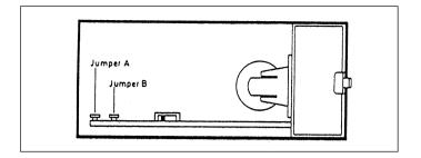
If the jumper B is connected, the Menu / Select key is locked; menu parameters can neither be printed nor modified.
