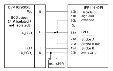
If the EOC pulse has a rising edge as in this example, it is applied to pin 19a. Pin 20a and pin 21a must be connected to each other to invert the EOC pulse.
