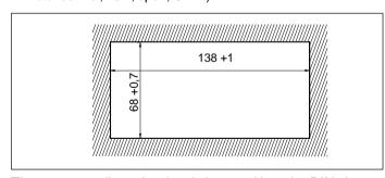
The paper reroll mechanism is inserted into the DIN size panel cutout from the front side and is clamped against the rear side of the switchboard using the mounting screws. The switchboard thickness must not exceed 12 mm.
