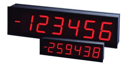
Large Displays OC57-RMS, OC100-RMS and OC125-RMS are 4 or 6 digit programmable instruments with up to 20'000 true increments and selectable inputs for various signals such as voltage from 0-200mV to 380V true RMS, currents from 20mA up to 10A true RMS or power up to 2300 W true RMS.
