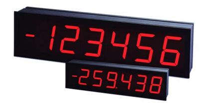
Large Displays OC57-RS, OC100-RS and OC125-RS are 4- or 6-digit programmable instruments with up to ±999999 display increments. They have inputs for RS232. RS485. RS422 and TTY serial data signals and can be ordered with 57mm, 100mm or 125mm large 7 segment display units. Customized displays are available upon request.
