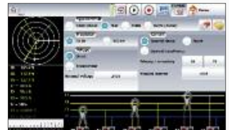
Setup menu with schematics to show how to connect the clamps.
