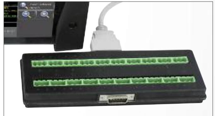
20 analogue channels board P/N: 902401000
