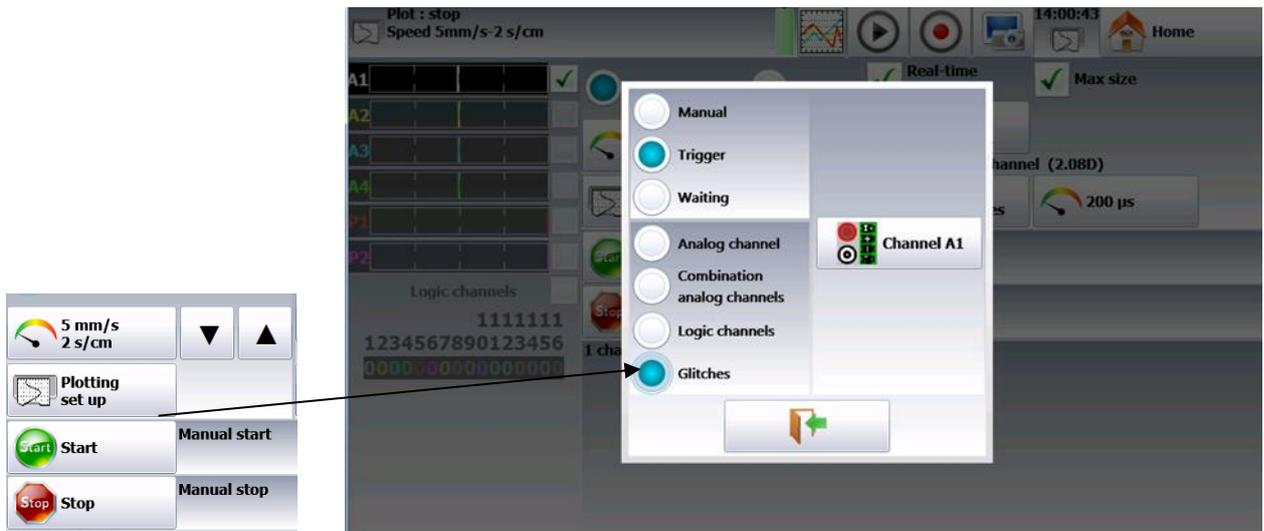
Trigger on Logic Channels
