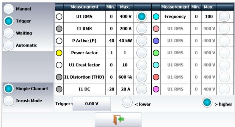
“Inrush” mod: the trigger occurs when the current is over a threshold with hysteresis.
