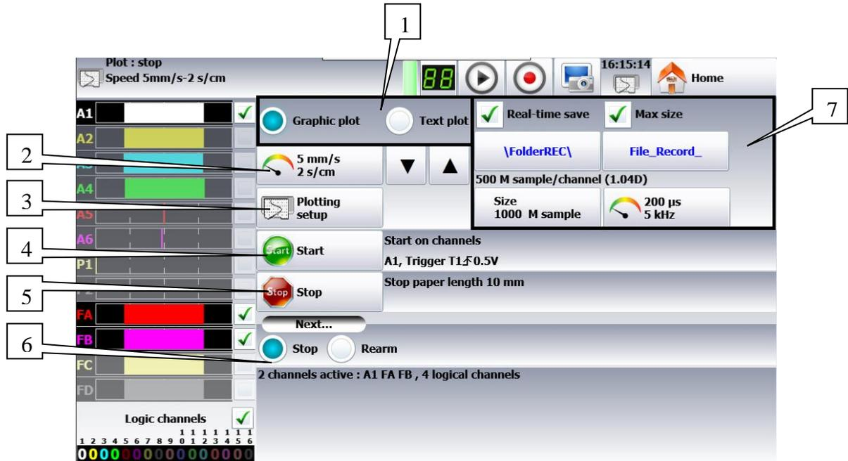
The screenshot shows the 'Plot : stop' interface. Callout 1 points to the 'Graphic plot' radio button. Callout 2 points to the '5 mm/s 2 s/cm' speed control. Callout 3 points to the 'Plotting setup' button. Callout 4 points to the 'Start' button. Callout 5 points to the 'Stop' button. Callout 6 points to the 'Next...' button. Callout 7 points to the 'File\_Record\_' button in the save settings panel.
