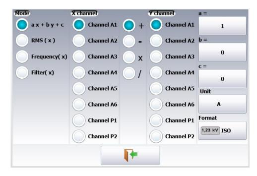
For the calculation of power, you will have: a(x\*y) + b with:x = channel A1operator = \*y = channel A2coefficient a = 1
