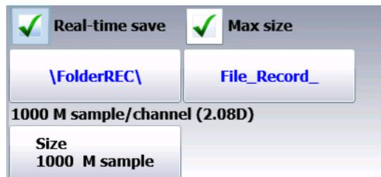
As soon as the record is launched, the device saves the samples into the file. The file closes when the data acquisition is done.
