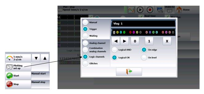
The 16 logic channels can be used in the trigger word:
