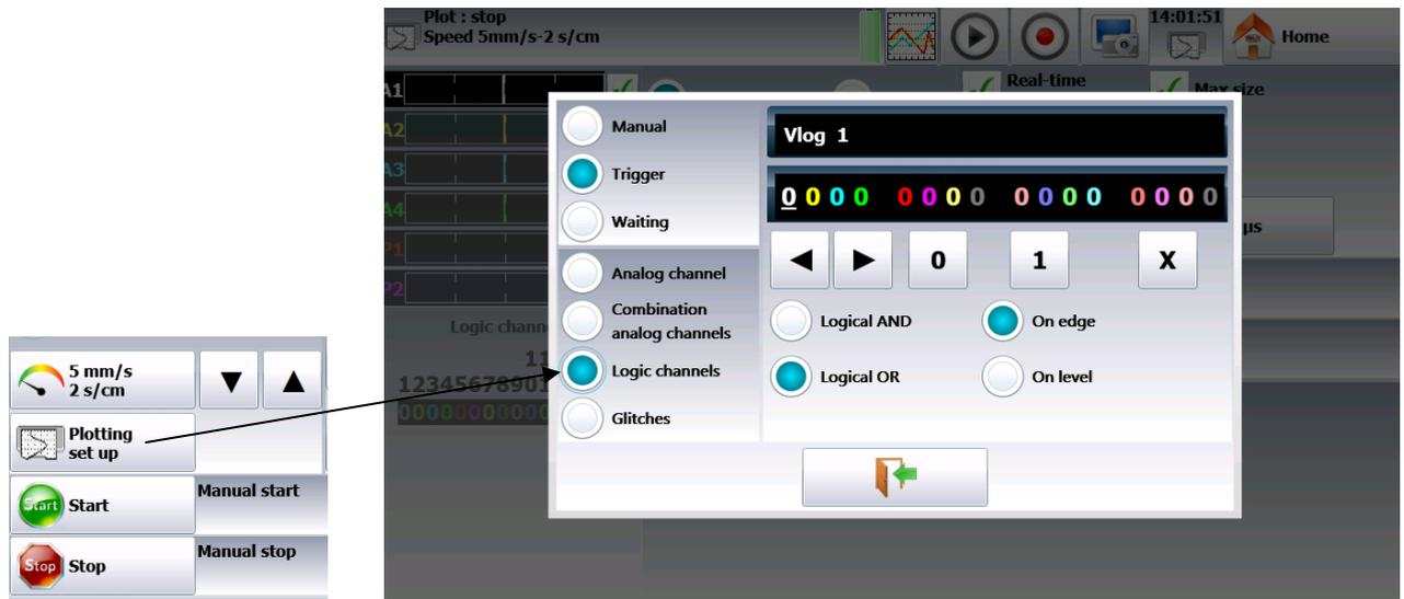
The 16 logic channels can be used in the trigger word:
