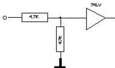
Non-connected inputs are 0V potential (level 0).
